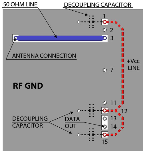
**Note:** Dotted elements must be placed on component side ( PCB side opposite to ground layer ).
