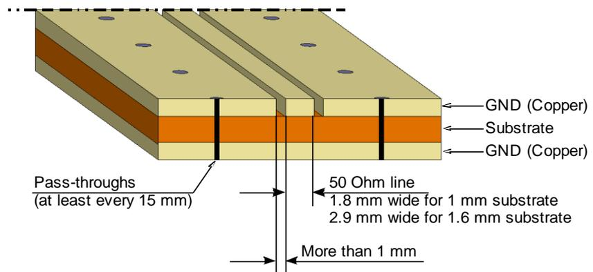
**Note:** the dimensions in the picture above are referred to a FR4 substrate PCB
