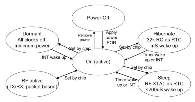
Once set up, the HF-BL200 power management algorithm will enter low-power states when possible, and wake up for advertising, connection and calibration activities as needed.
