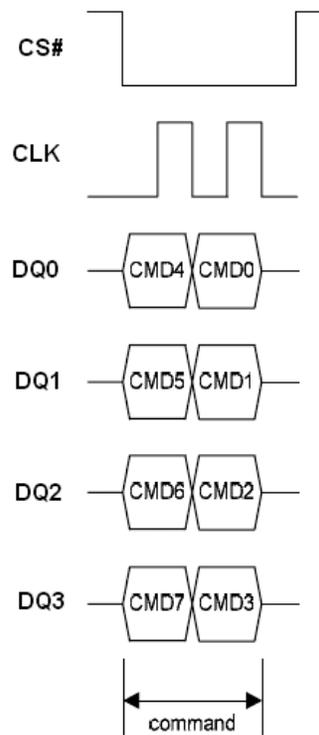
**Figure 35.1 Enter OTP Mode Sequence in QPI Mode**
