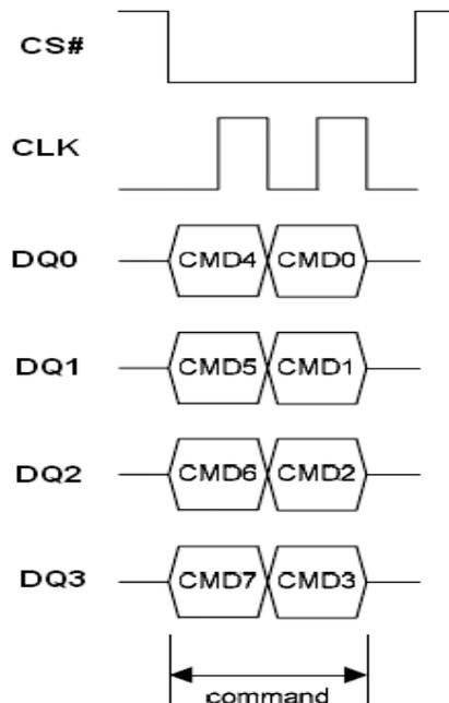
**Figure 29.1 Chip Erase Sequence in QPI Mode**
