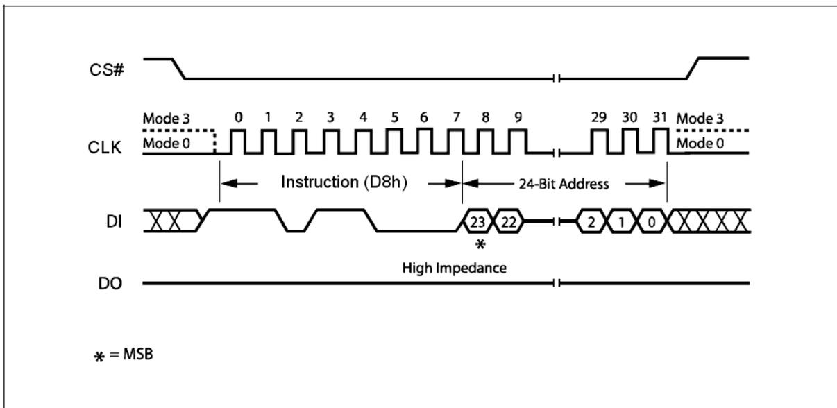
**Figure 28. 64KB Block Erase Instruction Sequence Diagram**
