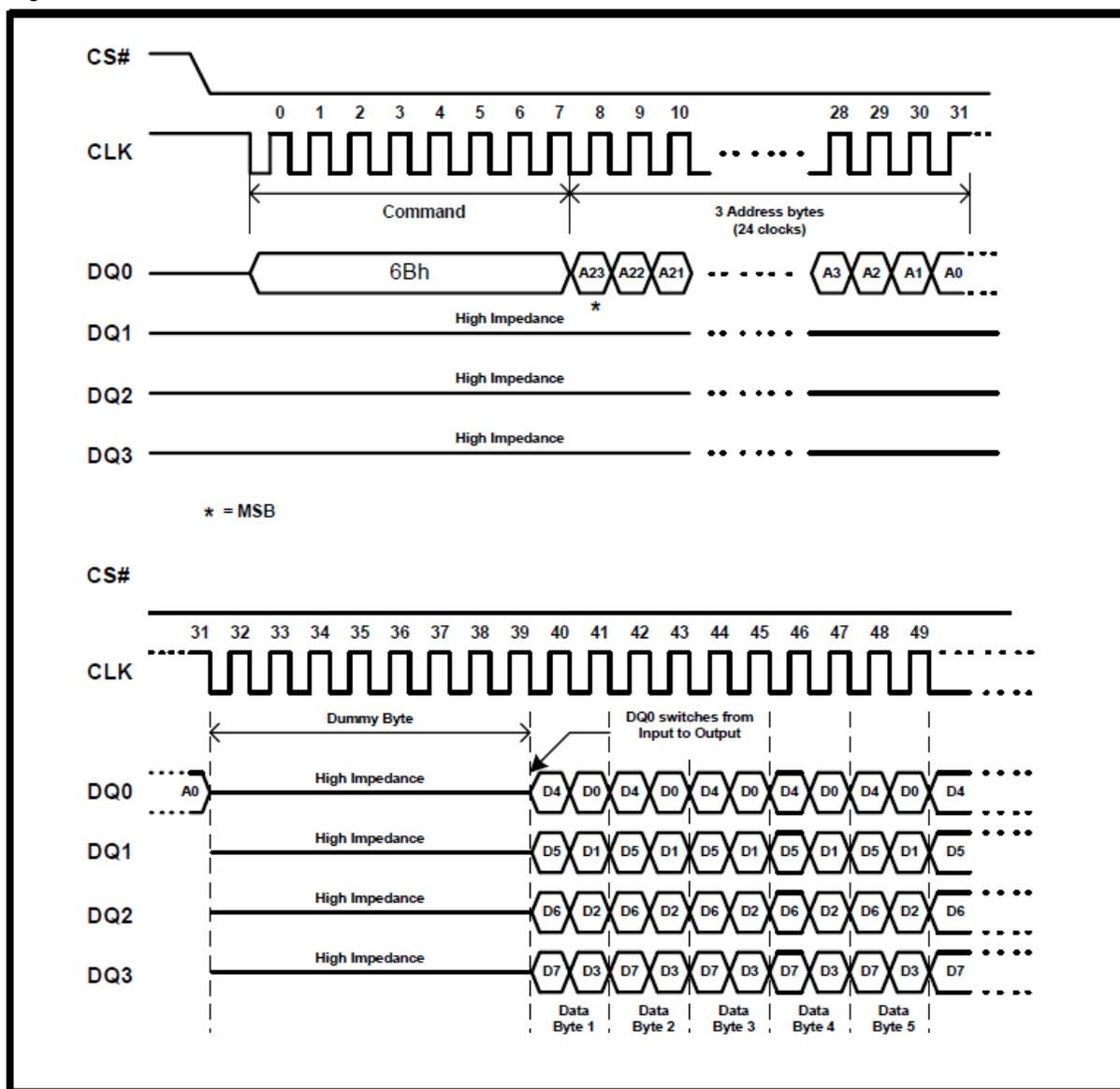
**Figure 20. Quad Output Fast Read Instruction Sequence Diagram**
