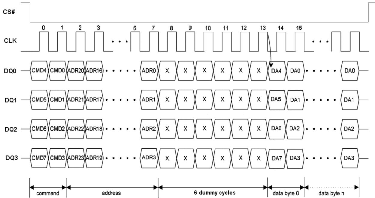
**Figure 15.1 Fast Read Instruction Sequence in QPI Mode**
