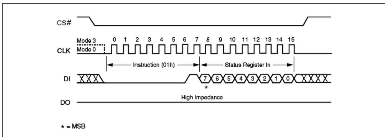
**Figure 13. Write Status Register Instruction Sequence Diagram**
