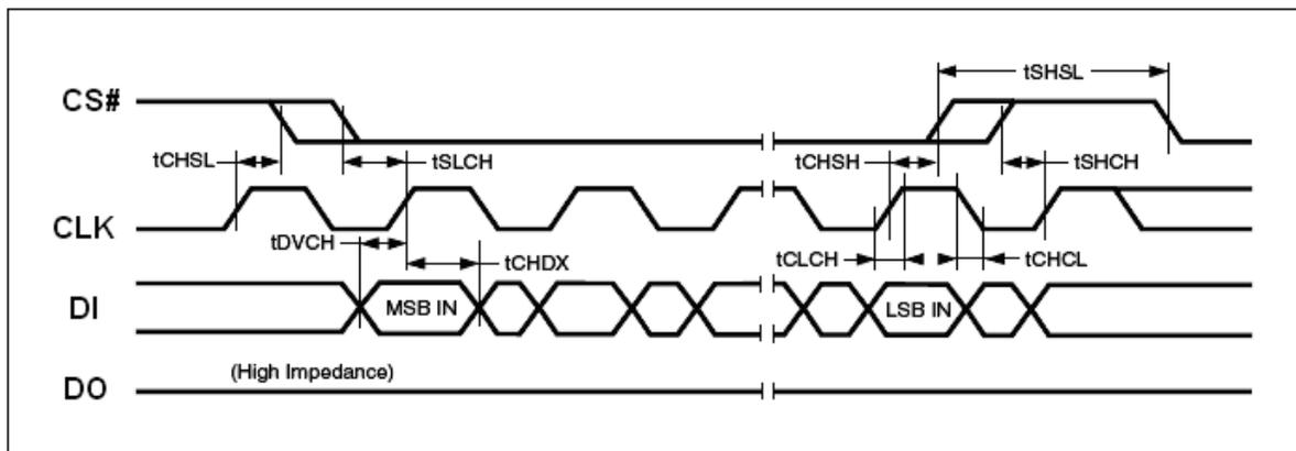
**Figure 40. Input Timing**
