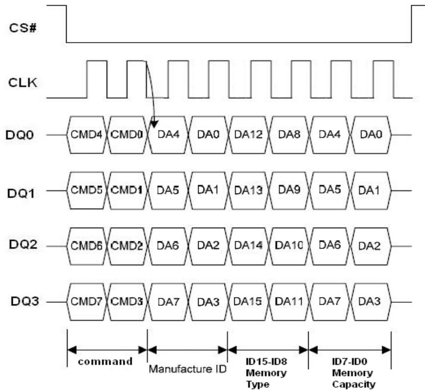
**Figure 34.1 Read Identification (RDID) in QPI Mode**
