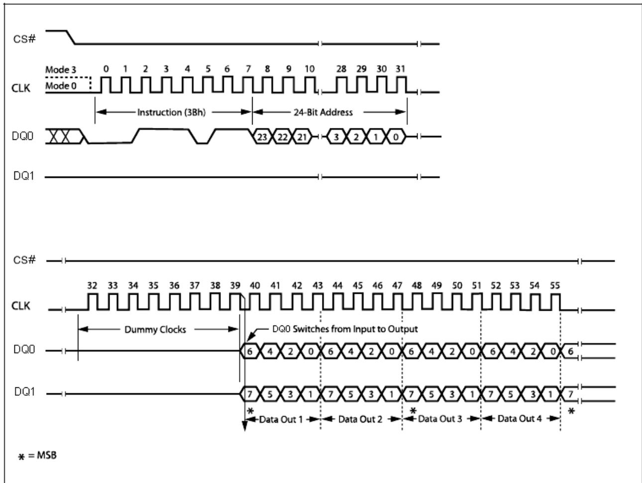
**Figure 16. Dual Output Fast Read Instruction Sequence Diagram**
