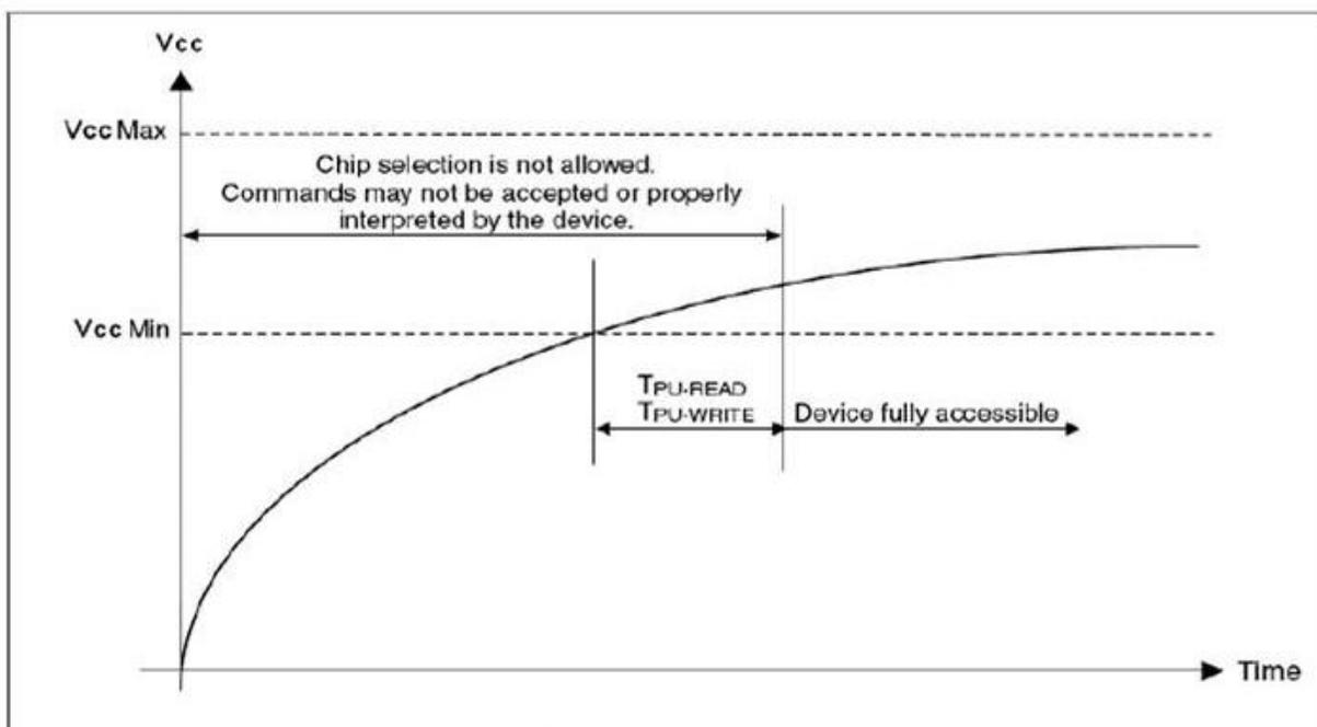
**Figure 37. Power-up Timing**
