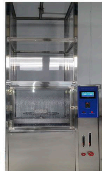
Testing under water jet
