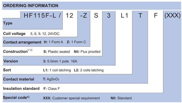
Notes: 1) We recommend flux proofed types for a clean environment (free from contaminations like H<sub>2</sub>S, SO<sub>2</sub>, NO<sub>2</sub>, dust, etc.). We suggest to choose plastic sealed types and validate it in real application for an unclean environment (with contaminations like H<sub>2</sub>S, SO<sub>2</sub>, NO<sub>2</sub>, dust, etc.).
