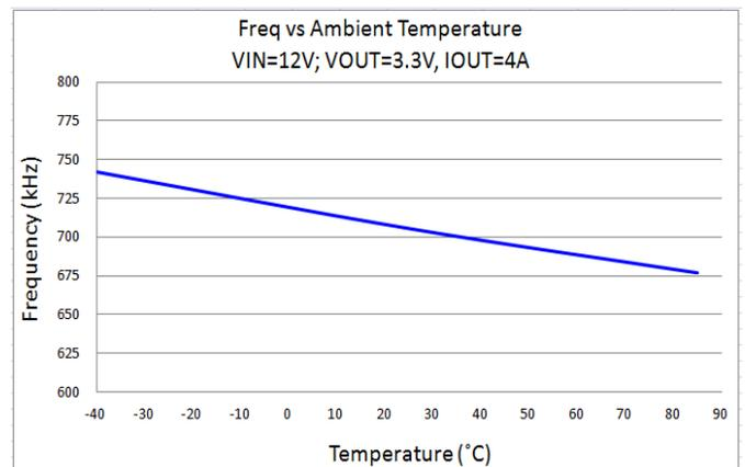
**Typical Performance Characteristics** (continued) (@T<sub>A</sub> = +25°C, V<sub>IN</sub> = 12V, V<sub>OUT</sub> = 3.3V, unless otherwise specified.)
