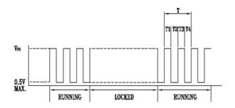
T=T1+T2+T3+T4=60/N(Sec) N:SPEED (RPM)
