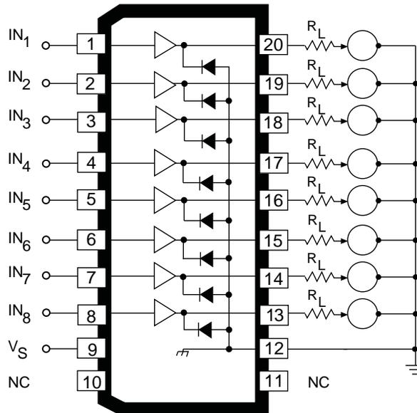
Pins 10 and 11 can float; other pins match discontinued 18-pin SOIC: 1 to 9 same, pins 12 to 20 match pins 10 to 18
