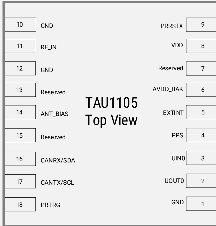
Figure 3 Pin assignment (top view)
