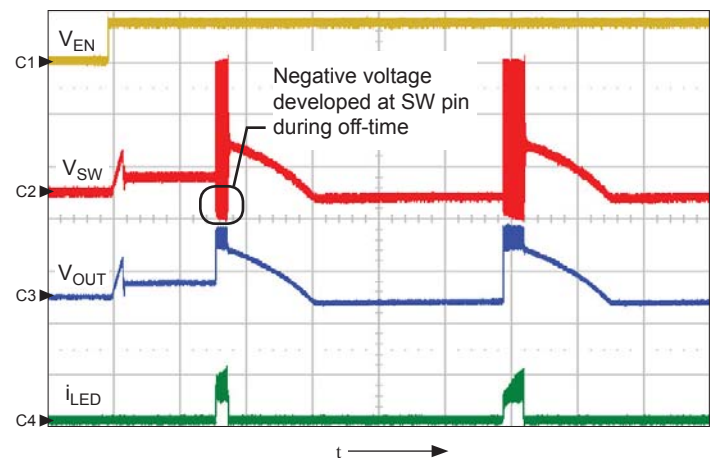
Figure 11. Startup waveform with a missing Schottky diode; shows Enable, V_{EN} (ch1, 5 V/div.), switch node, V_{SW} (ch2, 5 V/div.), output voltage, V_{OUT} (ch3, 5 V/div.), LED current, i_{LED} (ch4, 500 mA/div.), t = 100 \mu s/div.
