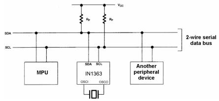
Data transfer can be started only when the bus is not busy. In the process of the data transfer, the data line should remain stable, while the cycle signal line is in the HIGH condition. Alterations of the data line conditions at that moment, when the cycle line is in the high condition, will be regarded as the control signals.
