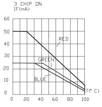
MAXIMUM FORWARD DC CURRENT VS, AMBIENT TEMPERATURE.
