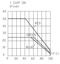
MAXIMUM FORWARD DC CURRENT VS, AMBIENT TEMPERATURE.
