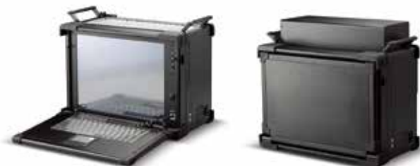
Top cover to protect PXI/cPCI modules and wirings
