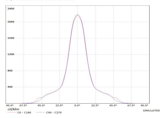
Luminaire: C12083\_Brooke-SCR-M C12083\_Brooke-SCR-M Lamps: 1 x Citizen CL-L330 1044lm 5000K 250mA
